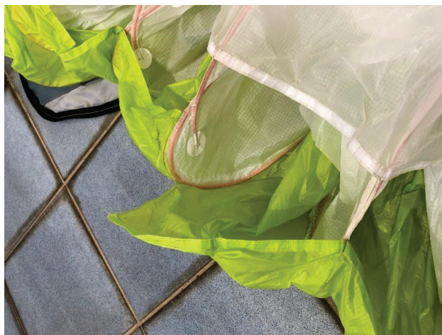
Figure 5: Damaged Canopy Leading Edge Cell Opening
